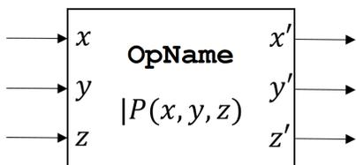
**Fig. 3.** Generic graphical notation for a deterministic, conditioned reversible operation  $\text{OpName}(x, y, z \mid P(x, y, z))$  on three state variables  $x, y, z$ , with an assumed precondition specified by the propositional function  $P(x, y, z)$ .
