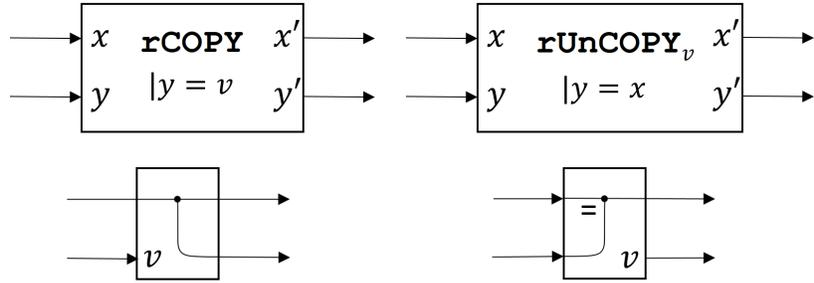
**Fig. 6.** (Left) Reversible copy of  $x$  onto  $y = v$ , top: standard notation, bottom: simplified symbol; (Right) Reversible uncopy of  $x$  from  $y$  back to  $v$ , top: standard notation, bottom: simplified symbol.
