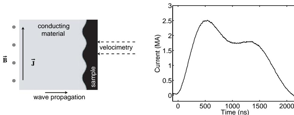
**Fig. 3.2.** Left: schematic setup in experiments planned for the Veloce device [10] to measure material strength using RT instability.  $\vec{J}$  denotes the current density vector and  $\vec{B}$  the magnetic flux density vector. Right: current pulse generated by Veloce.
