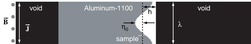
**Fig. 4.3.** Setup for ALEGRA simulations, showing current density  $\mathbf{J}$  imposed by boundary conditions; perturbation wavelength  $\lambda$  and initial amplitude  $\eta_0$ ; and sample thickness  $h$ .
