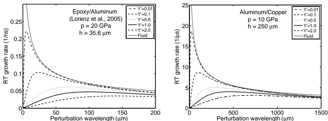
**Fig. 2.1.** Rayleigh-Taylor growth rates  $\gamma$  computed for (left) the conditions of Lorenz *et al.* (2005) [5] and (right) an aluminum-copper interface accelerated at 10 GPa, using the model of Colvin *et al.* (1998) [1], given in equation 2.6.
