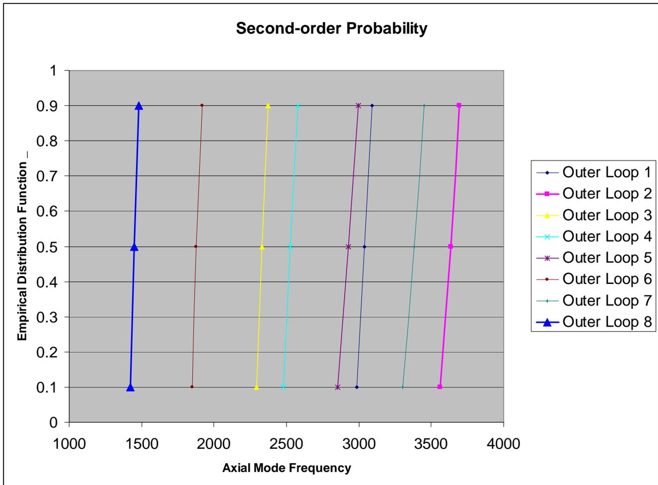
Figure 16. Second-order Probability Analysis for Axial Mode
